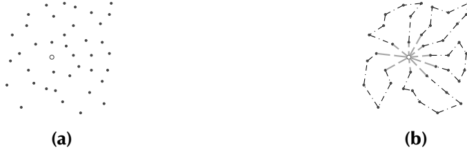
Figure 3: A CVRP example with n = 40 and k = 5 . Given the dispersed points shown in (a), CVRP asks to find the routes presented in (b).
